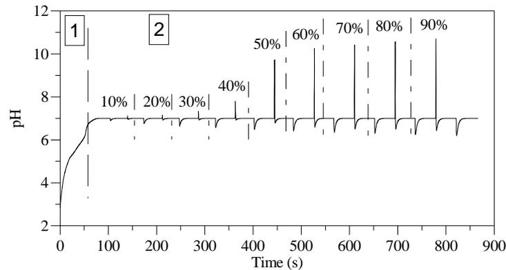
Figure 3. – Variation of pH vs time during the system start up and after acidic concentration perturbations. Zone 1: Start up. Zone 2: Acidic concentration perturbations. The % is referred to the steady state value before perturbation.
