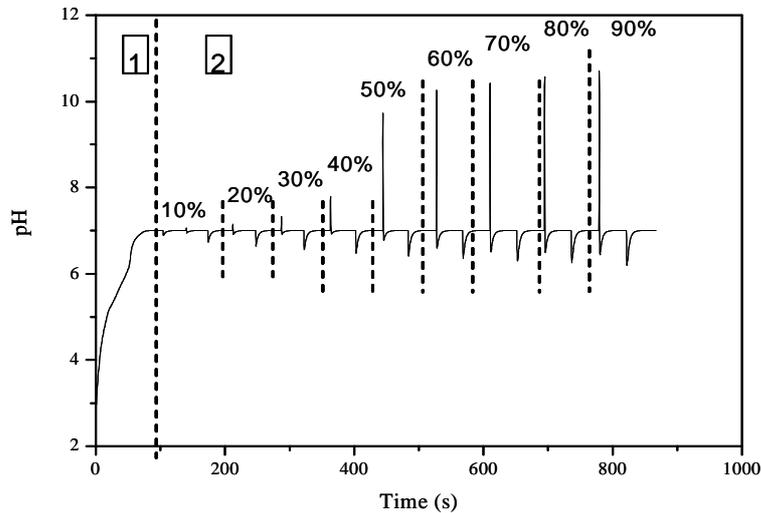
Figure 4. – Variation of pH vs time during the system start up and after acidic flow rate perturbations. Zone 1: Start up. Zone 2: Acidic flow rate perturbations. The % is referred to the steady state value before perturbation.
