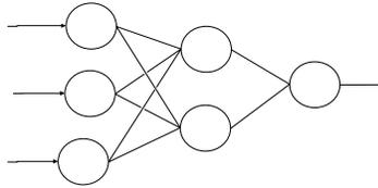
Fig. 1. Schematic of a multi-layer feed forward neural network model
