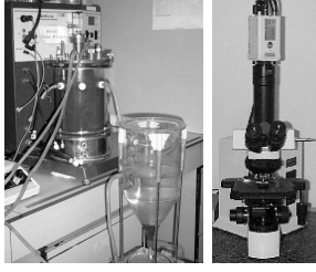
Figure 1: Left: lab-scale activated sludge system. Right: microscope (Olympus BX51) and video camera (Sony DXC-950P) used for daily capturing of activated sludge images.
