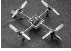
Figure 1: A prototype X4-flyer.
