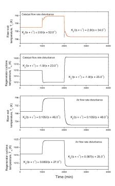
Figure 1: Step identification for a FCC unit for control design purposes.
