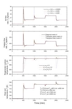
Figure 2: Closed-loop performance of three decentralized control configurations for a FCC unit.
