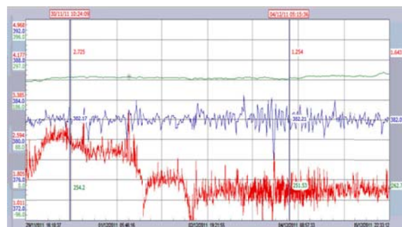
Figure 20: DCS snap-shot highlights O 2 % reduction on real system
