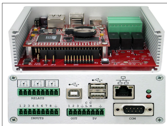
Fig. 1. Front and inside views of the embedded system used in the project as a MPC controller
