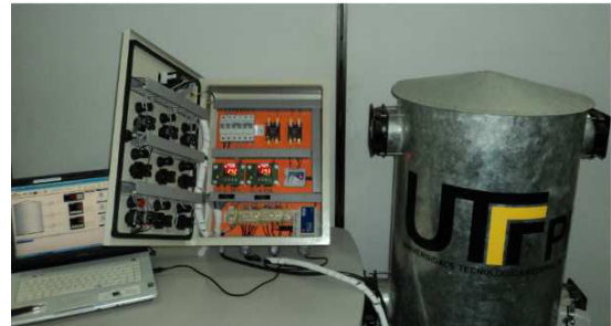
Fig. 4. Picture of the laboratory testbed used in the experiments. The apparatus comprises the grain silo prototype that stored wheat infested by R. dominica , the electrical control panel that implements the control of temperature inside the silo, and a computer to collect and save all of the required data.
