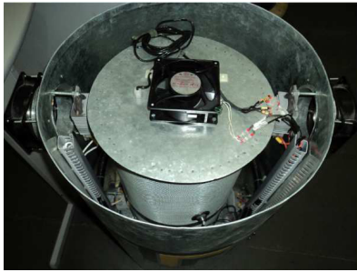
Fig. 2. A view from the top of the grain silo prototype (picture taken without the roof).
