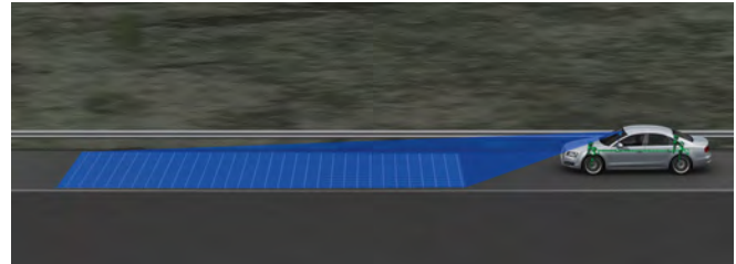
Fig. 1. Vehicle with active suspension and preview information
