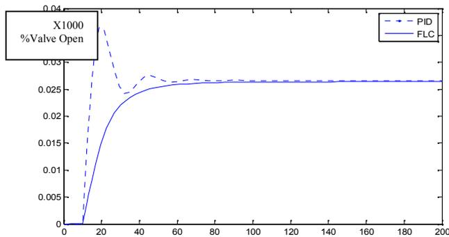
Figure 13: Control Action of PID & FLC; Vs Time (Sec), for SP=0.3.
