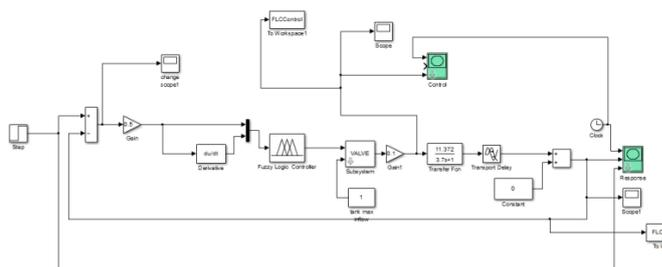
Figure 6: Flow process with FLC Controller.
