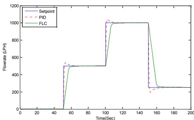
Figure 18: Response of FLC&PID; Flow Rate (LPH) Vs Time (sec), SP1=0, SP2=500, SP3=1000, SP4=250.
