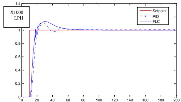
Figure 16: Response of PID & FLC; Vs Time (Sec), for SP=1
