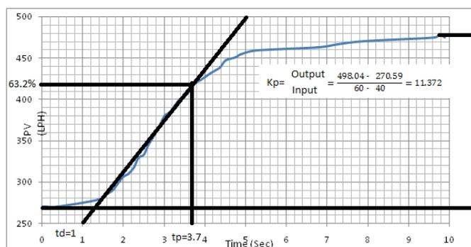
Figure 8: Step response in flow rate for input step change from 40 - 60%.
