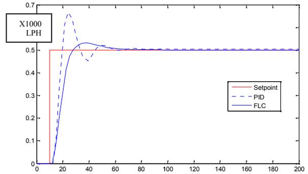
Figure 14: Response of PID & FLC; Vs Time (Sec), for SP=0.5
