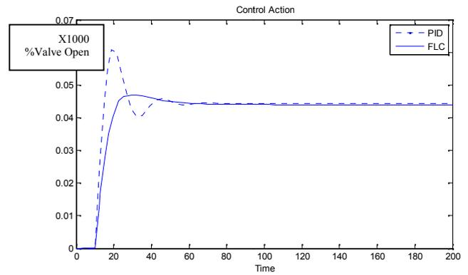
Figure 15: Control Action of PID & FLC; Vs Time (Sec), for SP=0.5.
