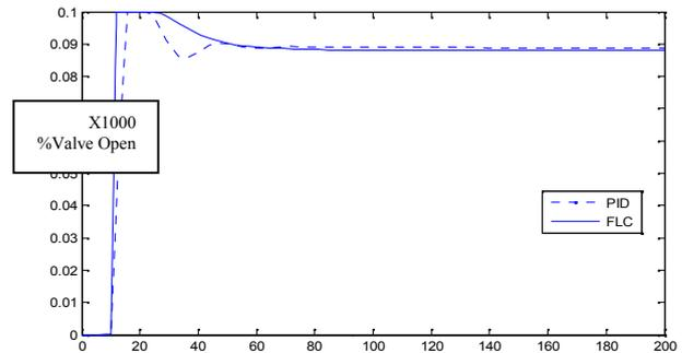
Figure 17: Control Action of PID & FLC; Vs Time (Sec), for SP=1 (on Y-axis: 100% valve open is Upper Limit).
