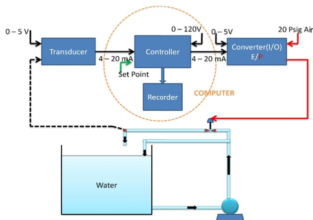
Figure 3.1: Schematic diagram of Flow Process Station
