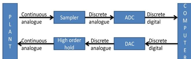
Figure 1: Plant to Computer Signal Flow
