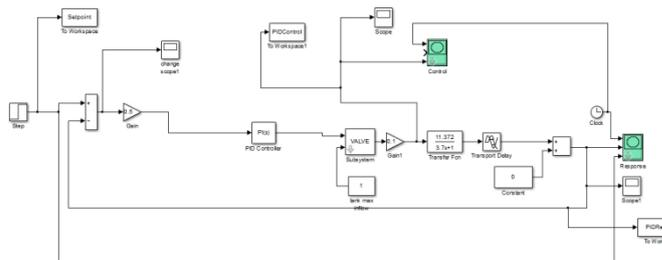
Figure 5: Flow process with PID Controller.
