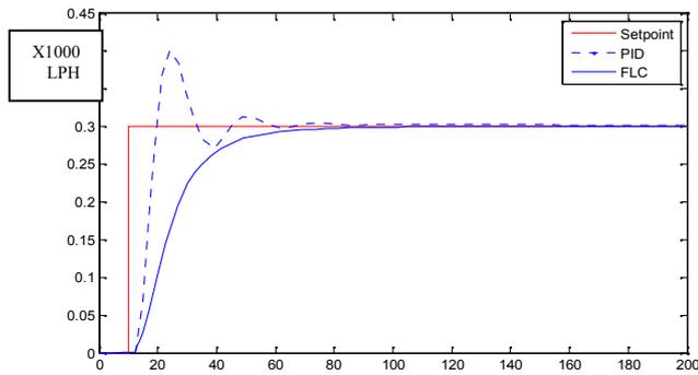
Figure 12: Response of PID & FLC; Vs Time (Sec), for SP=0
