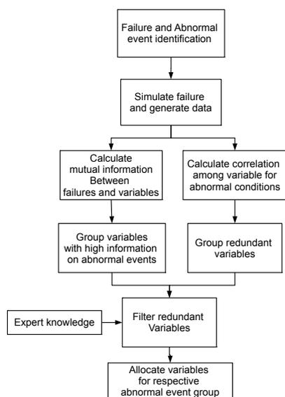
Fig. 1. Methodology for grouping variables to assign alarms
