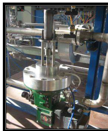
Fig. 2. Picture of the modified control valve (DVC5020F type).
