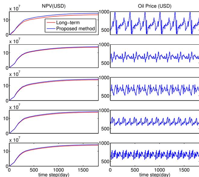
Fig. 7. Comparison between the NPV from the long-term optimization and the developed method for different oil price scenarios
