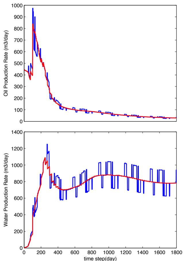
Fig. 8. Comparison between the production rate from the long-term optimization (red line) and the developed method (blue line) for the first oil price scenario
