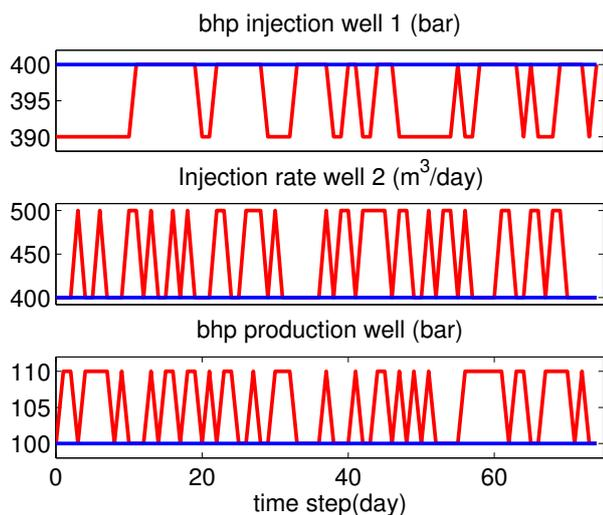
Fig. 5. First 75 days of exciting control actions (red line) and long-term optimization solution (blue line)
