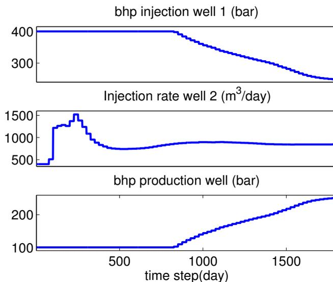
Fig. 4. Solution of the long-term optimization problem by applying the line search method, which uses adjoints to calculate the gradient.
