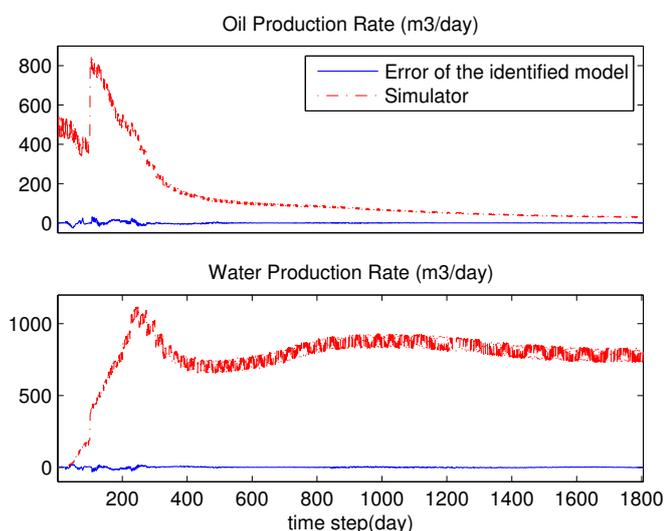
Fig. 6. Comparison between the liquid production rates from the simulator and the error of the identified model
