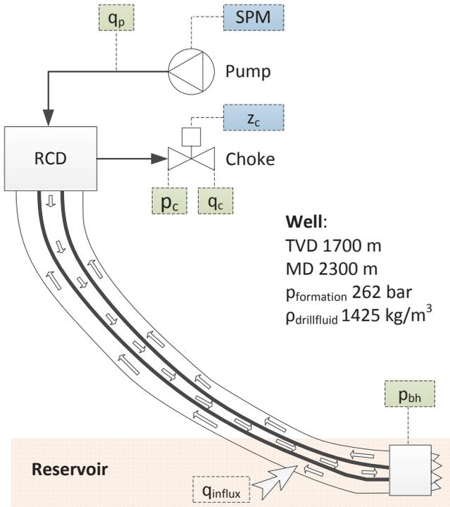
Fig. 1. Illustration of the well.
