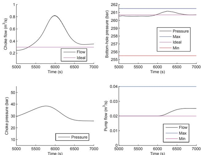
Fig. 7. Disturbance rejection of gas bubble.
