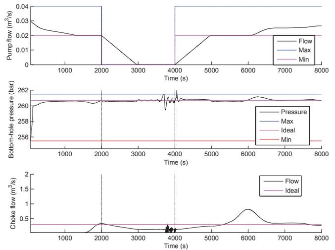
Fig. 5. Connection scenario with low ideal return flow.
