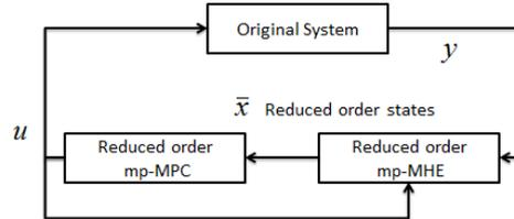
Figure 1: Schematic of simultaneous reduced order mp-MHE/MPC
