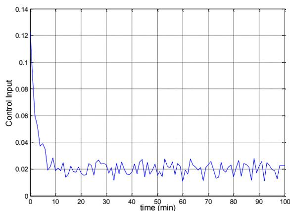
Figure 9: Evolution of the control input variable in the case of high measurement noise.
