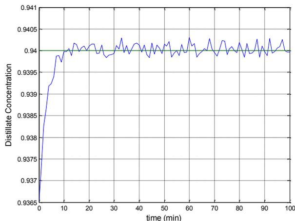
Figure 8: Close loop simulation of a set-point change operated through simultaneous mp-MHE and mp-MPC in the case of high measurement noise.
