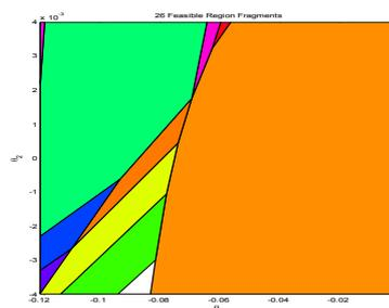
Figure 10: Critical regions for the mp-MPC controller implemented simultaneously to mp-MHE
