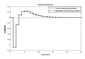
Fig. 3. Impulse response of identified model
