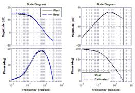
Fig. 2. Bode plots of the plant (left) and closed loop system (right)
