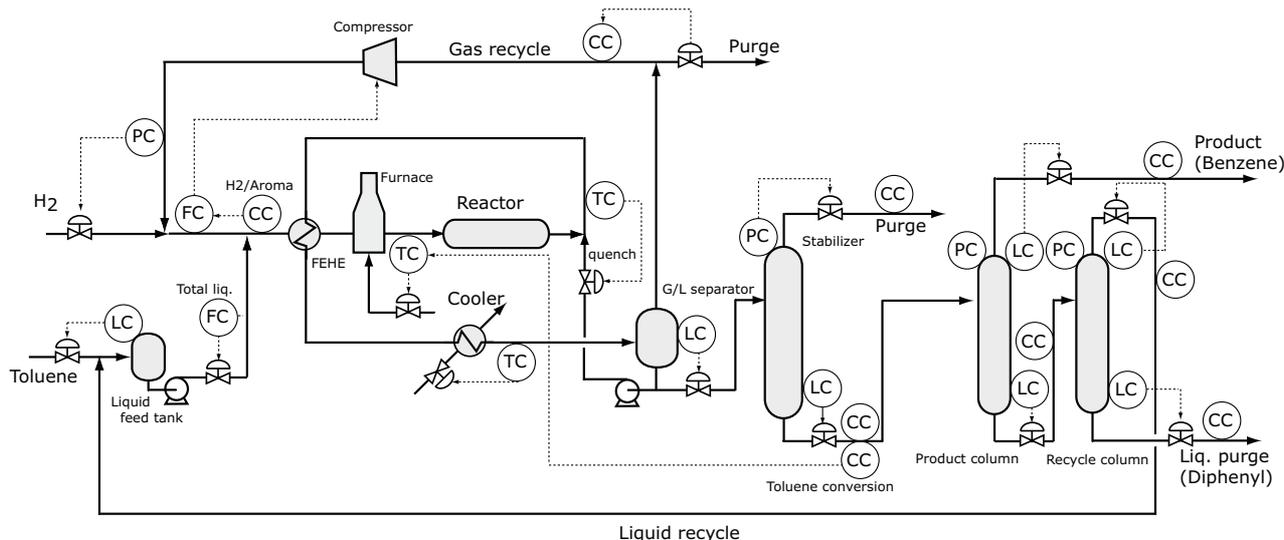
Fig. 2. The HDA process flow diagram with regulatory control loops
