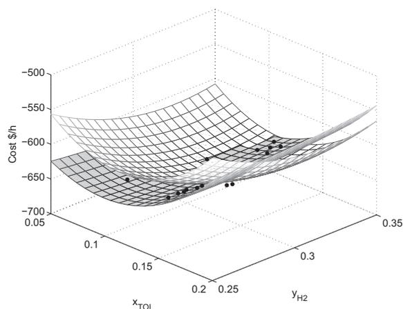
Fig. 8. Comparison of the cost models obtained from data with different numbers of sampling points. Shaded surface: 100 sampling points. Non-shaded surface: 30 sampling points.
