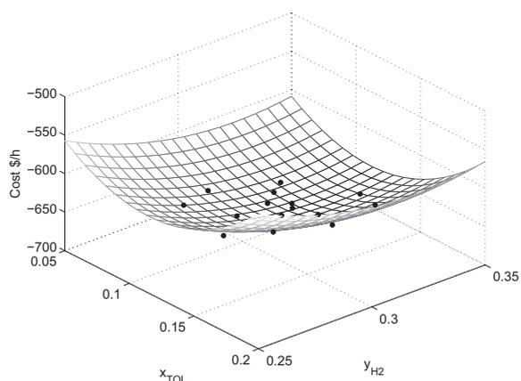
Fig. 7. Response surface model for the operation cost
