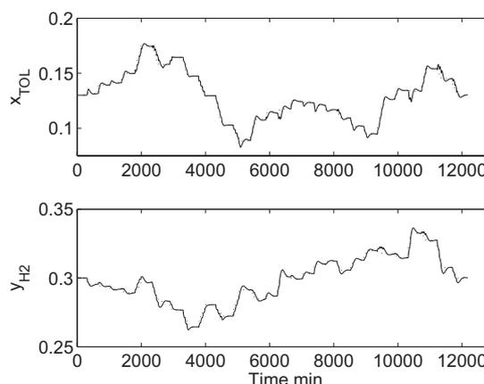
Fig. 4. Time plots of the independent variables. Dotted: setpoint, solid: actual.
