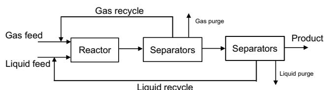
Fig. 1. Reactor/separators system with gas and liquid recycle streams
