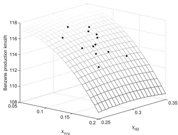
Fig. 5. Response surface for the benzene production. The dots are the sampling points.
