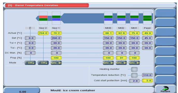
Fig. 5. Screen shot of Multi model based PID controller
