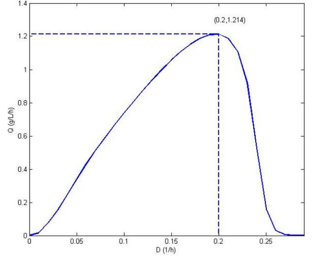
Fig. 2. Effect of the dilution rate on the productivity
