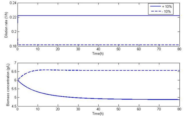
Fig. 3. Open loop for  $\pm 10\%$  change in dilution rate
