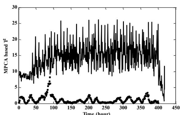
Figure 4: Modified MPCA based control charts for a ramp fault in aeration rate
