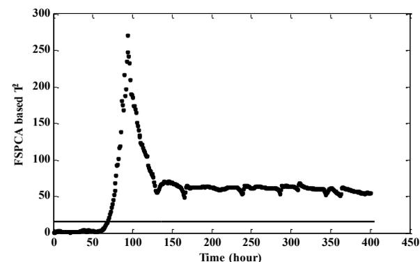
Figure 5: The proposed FSPCA based control charts for a ramp fault in aeration rate
