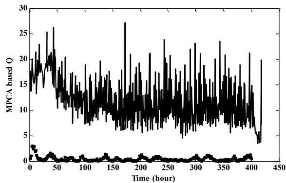
Figure 2: Modified MPCA based control charts for a ramp fault in agitator speed
