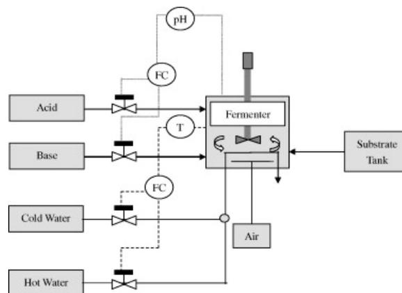
Figure 1: The fed-batch penicillin fermentation process
