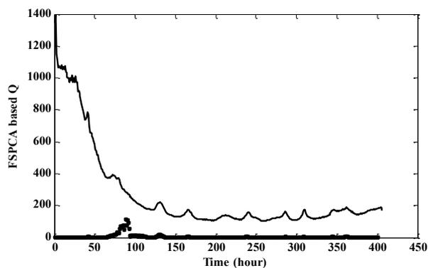
Figure 3: The proposed FSPCA based control charts for a ramp fault in agitator speed
