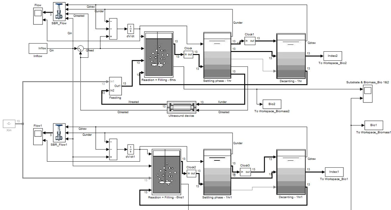
Fig. 2. Simulating implementation of SBR systems: Lower: control SBR Bio1 and upper: US treated SBR Bio2.
