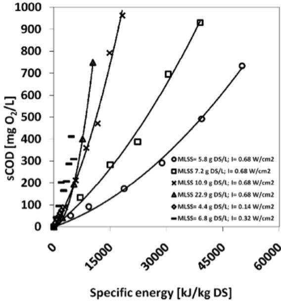
Fig. 3. sCOD change at different initial dry MLSS concentrations (4.4 – 22.9 g DS/L) and varying ultrasonic intensity values (0.14 – 0.68 W/cm<sup>2</sup>).
