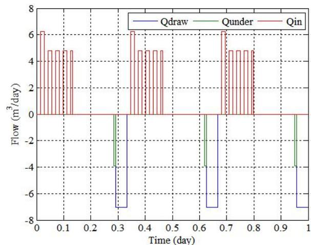
Fig. 7. Flow pattern during 1 cycle in SBR Bio2 at Mechelen-Nord.
