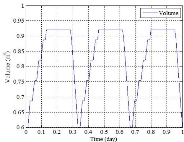
Fig. 8. Volume pattern during 1 cycle in SBR Bio2 at Mechelen-Nord.
