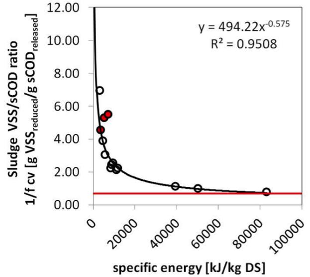
Fig. 4. Sludge sCOD/MLVSS ratio as a function of specific energy. Training and external validation sets are differentiated by open (o) and solid (•) circles, respectively.
