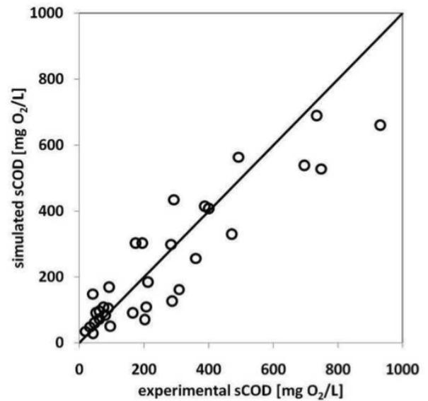
Fig. 5. Relation between simulated and experimental data for sCOD release in the supernatant liquid.
