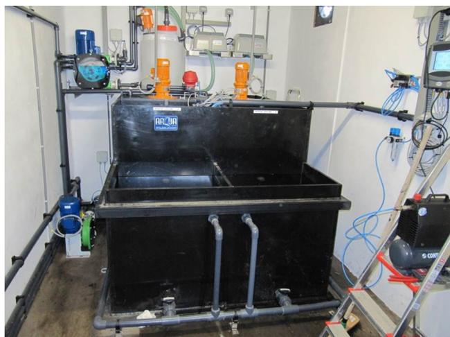
Fig. 1. The SBR pilot plant of this study.
