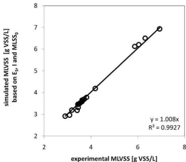
Fig. 6. Relation between simulated data and true data for MLVSS concentration. Training and external validation sets are differentiated by open (o) and solid (●) circles, respectively
