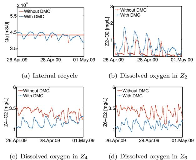
Fig. 8. Spring Scenario: Internal recycle flow-rate (a) and dissolved oxygen set-points in second (b), fourth (c) and sixth (d) zone of the bioreactor.
