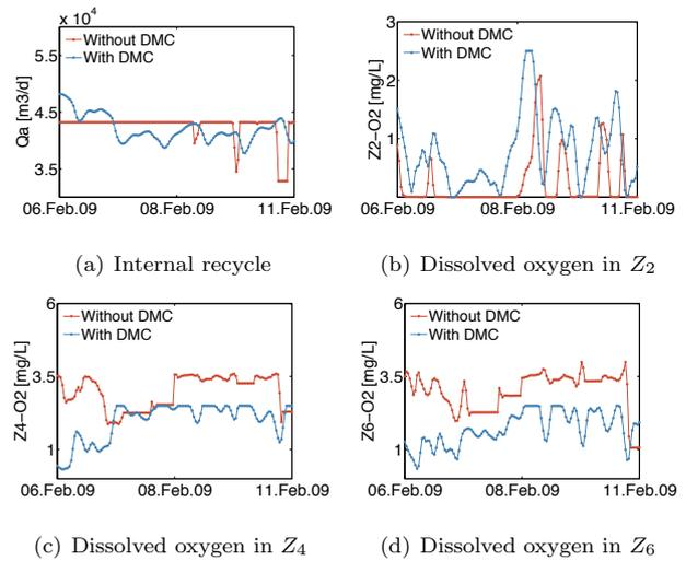
Fig. 7. Winter Scenario: Internal recycle flow-rate (a) and dissolved oxygen set-points in the second (b), fourth (c) and sixth (d) zone of the bioreactor.
