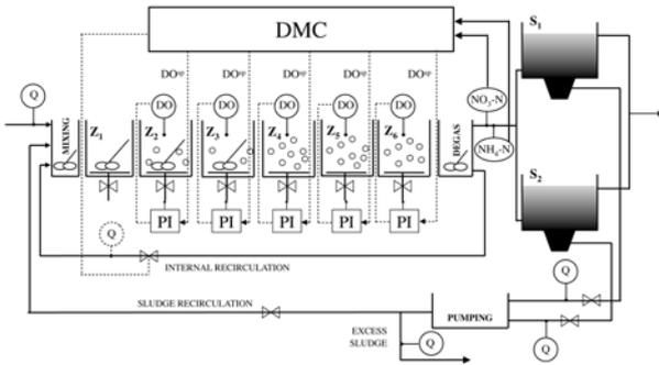
Fig. 5. DMC configuration for the activated sludge process of the Viikinmäki wastewater treatment plant.
