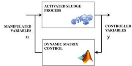
Fig. 4. Link between the process (GPS-X) and the controller (Matlab) in the simulation loop.
