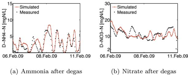
Fig. 2. Winter scenario: Simulation results comparison for ammonia (a) and nitrate (b) after the degas.
