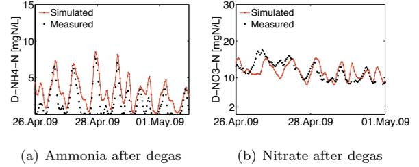
Fig. 3. Spring scenario: Simulation results comparison for ammonia (a) and nitrate (b) after the degas.
