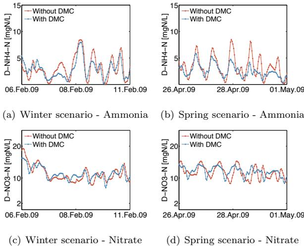
Fig. 6. Comparison of ammonia and nitrate concentrations after degas during winter, (a) and (c), and spring (b) and (d).
