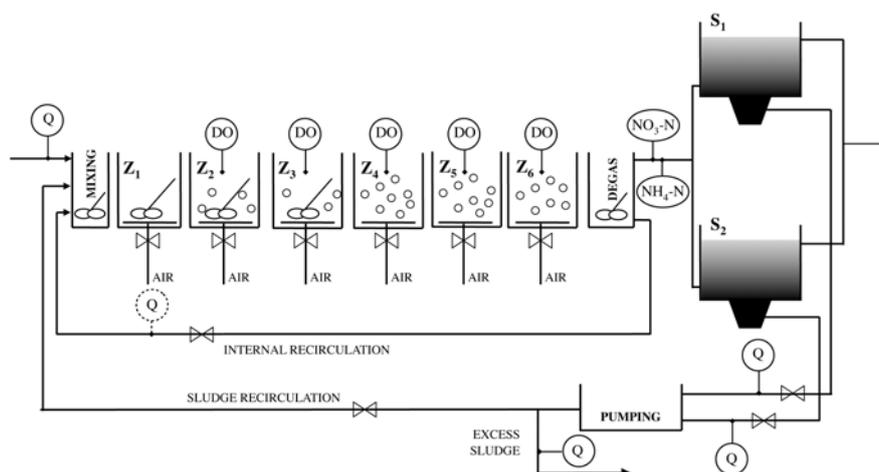
Fig. 1. A schematic of the activated sludge process of the Viikinmäki wastewater treatment plant.
