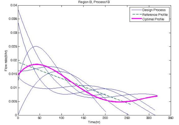
Figure 3: Some of the Feeding Profiles in Domain B for Process #13, along with the Center Point Reference Profile and the Calculated Optimal one
