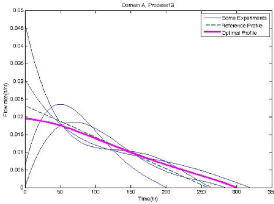
Figure 2: Some of the Feeding Profiles in Domain A for Process #13, along with the Center Point Reference Profile and the Calculated Optimal one
