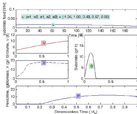
Figure 5: The Time Evolution of the State and Input Variables of the Optimum Operation for Process 13 in Domain B
