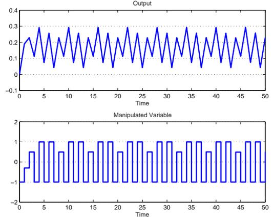
Fig. 4. MPC controller for Example 1, ( $y_{set} = 0.2$ ,  $p = 20$ ,  $m = 10$ )
