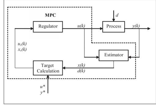
Fig. 1. Typical architecture of MPC controller.
