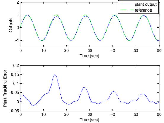
Fig. 2. Plant tracking response with parameter disturbance ( $\alpha_2$  changes from 1 to 1.5 at  $t = 5s$ )
