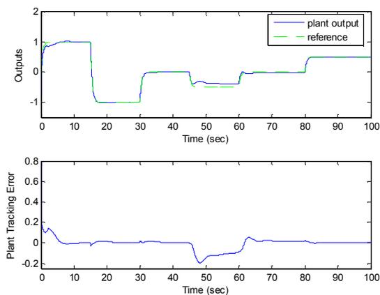
Fig. 5. Plant tracking response with parameter disturbance ( $\alpha_1$  changes from 1 to 1.5 at  $t = 44s$ )
