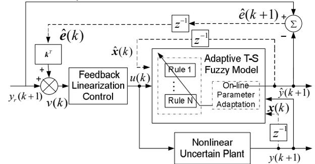
Fig. 1 Adaptive control based on T-S fuzzy model
