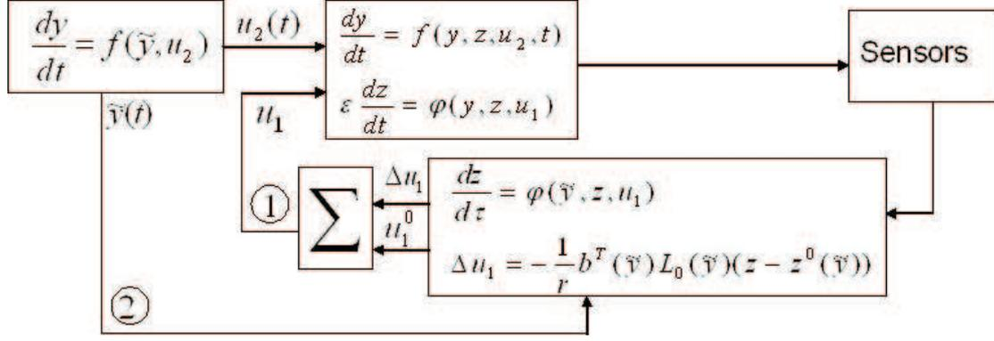
Fig. 1. Scheme of the two level control for the singularly perturbed system.
