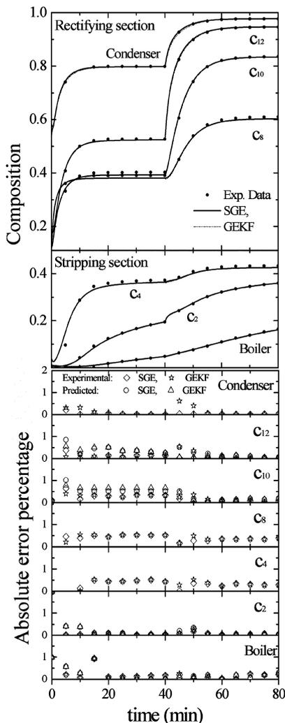
Fig. 5. SGE and GEKF estimation with partial innovation
