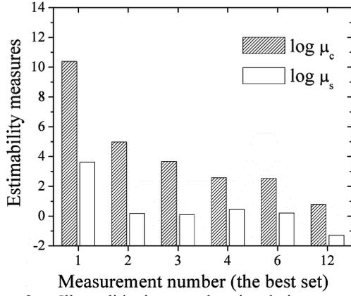
Fig. 3. Ill-conditioning and singularity measure dependencies on the number of optimally placed sensors.
