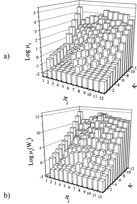
Fig. 2. Single-sensor singularity measure ( $\mu_s$ ) dependency on sensor location ( $\pi_i$ ) and estimation order ( $\kappa$ ), at  $t = 40$  min, using estimation (a) and Grammian (b) matrices.
