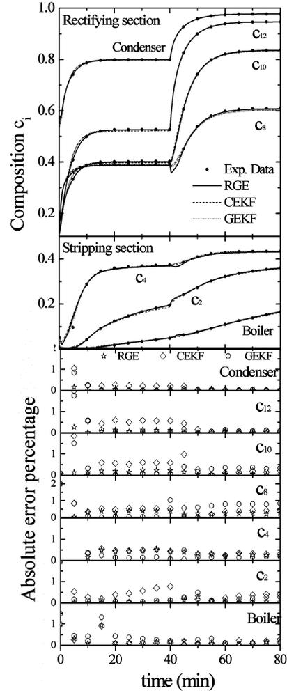
Fig. 4. *SGE*, *CEKF* and *GEKF* estimation with complete innovation.
