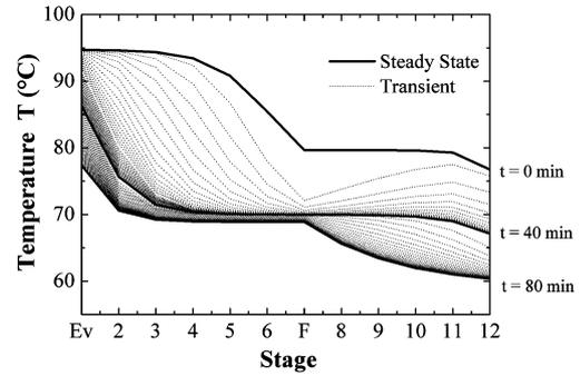
Fig. 1. Experimental temperature profiles evolution
