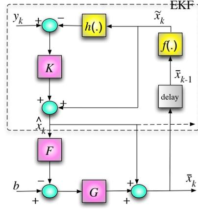
Fig. 1. Constrained extended Kalman filter
