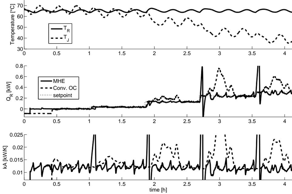
Fig. 1. Application of the MHE and conventional oscillation calorimetry to an experiment performed in a 1 l glass reactor
