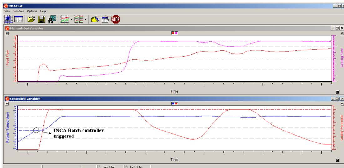
Fig. 6. Qualitative view of the control behavior of the INCA<sup>®</sup> batch controller on the batch process at the Air Products and Chemicals Inc. plant. Cooling and quality constraints are depicted as dash-dotted lines.
