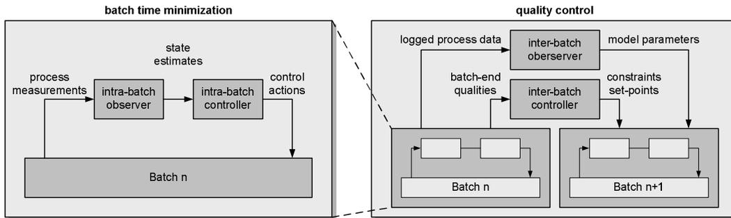
Fig. 4. Cooperation between inter- and intra-batch observers and controllers for batch time reduction and end-quality control.
