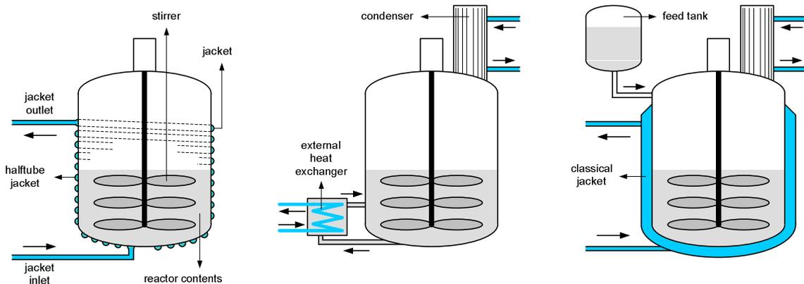
Fig. 1. Different types of batch reactors. **Left:** batch reactor with half-tube jacket. **Middle:** Batch reactor with external heat exchanger and condenser. **Right:** Fed-batch reactor with condenser and classical jacket.
