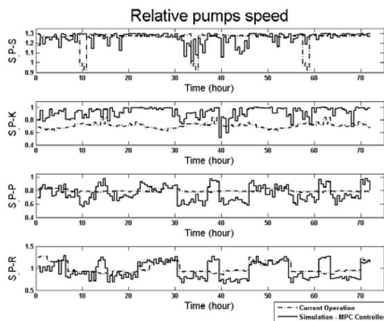
Fig.2. Relative speeds of the pumps Sieradzka, Kolibki, P1 and Reda
