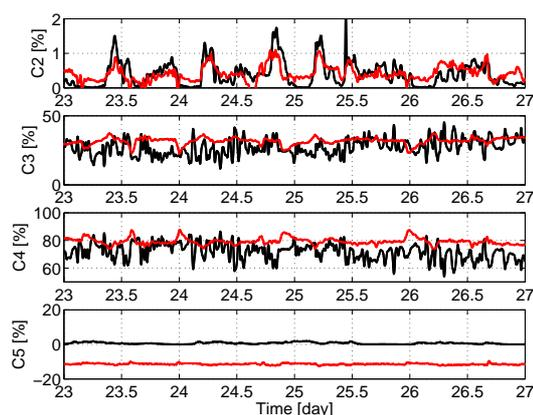
Fig. 1. LPG case study: training results (one week) of the GDS C2 sensor (grey line). Analyzer measurements: black line.
