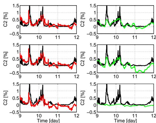
Fig. 2. LPG case study: validation results of the GDS (left) and PRESTO (right) C2 sensor. Model trained with 1 month (grey line, top), 1 week (grey line, center) and 1 day data (grey line, bottom). Analyzer measurements: black line.
