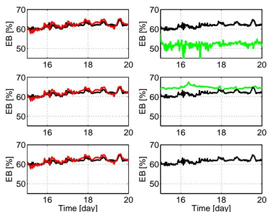
Fig. 4. SM case study: validation results of the GDS (grey line, left) and PRESTO (grey line, right) top EB concentration. Models trained with 1 month (top), 1 week (center) and 1 day (bottom) data. Analyzer measurements: black line.
