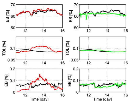
Fig. 3. SM case study: training results of the GDS (grey line, left) and PRESTO (grey line, right) top EB concentration (top), bottom TOL concentration (center) and bottom EB concentration (bottom) sensors. Models trained with 1 month data. Analyzer measurements: black line.
