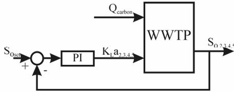
Fig. 3. Control scheme of oxygen PI control.
