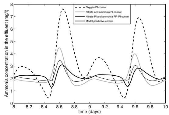
Fig. 7. Comparison of effluent ammonia concentrations.
