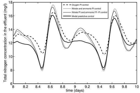
Fig. 8. Comparison of effluent total nitrogen concentrations.
