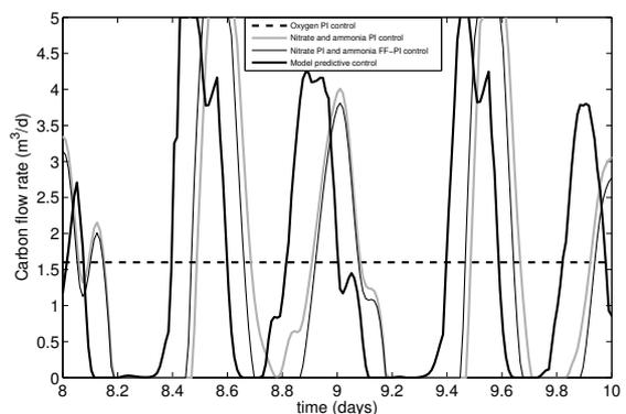
Fig. 10. Comparison of external carbon flow rates.
