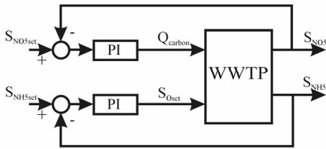
Fig. 4. Control scheme of nitrate PI and ammonia PI control.
