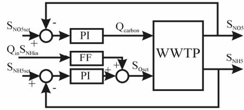
Fig. 5. Control scheme of nitrate PI and ammonia FF-PI control.
