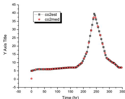
Fig. 3. CO<sub>2</sub> concentration: estimate and measure states.
