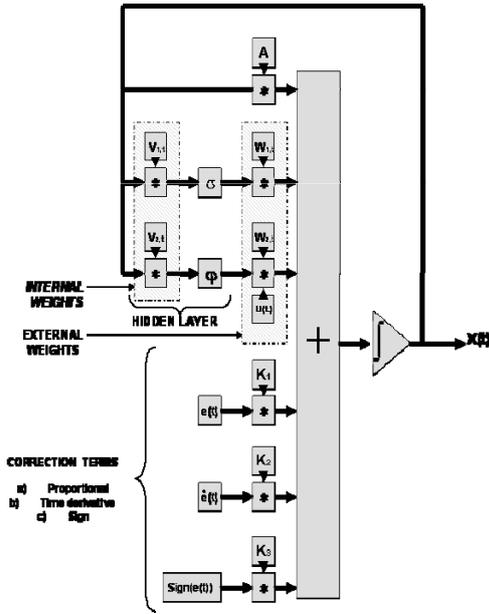
Fig. 1. Block diagram of the Neuro Observer added with the correction terms.
