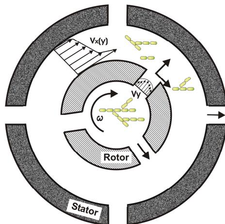
Fig. 8. Schematic representation of a rotor-stator device for inline disruption of moss treads and pellets during a suspension culture in a pilot photobioreactor. A focused cut of the moss is produced by the incidence of two velocity gradients mainly at the exit of the rotor channels.
