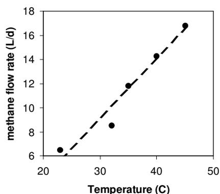
Fig. 2. The effect of temperature on the methane production rate at an OLR of 55 g COD d<sup>-1</sup>
