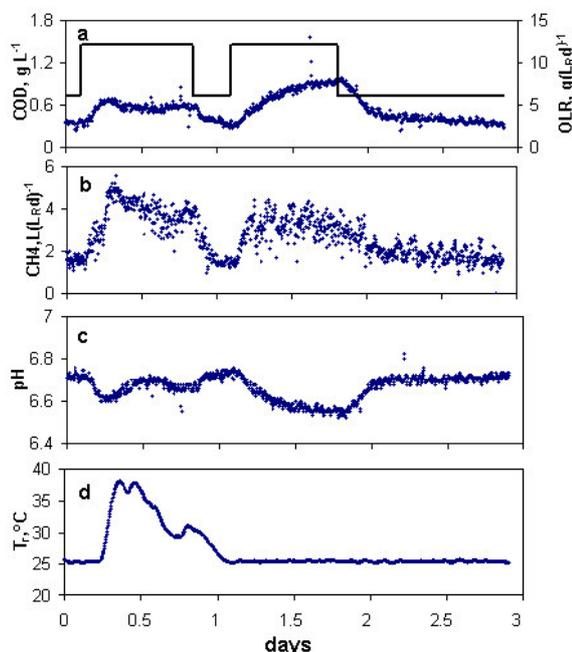
Fig. 3. Dynamics of key process parameters (a-d) and temperature (e) in a 10 L reactor during feedback control (0-1.1 day) and open-loop (1.1-3 day) experiments.
