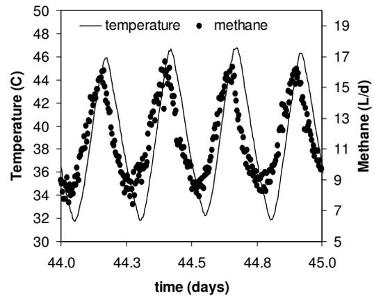
Fig. 1. Reactor operation at an OLR of  $55 \text{ g COD d}^{-1}$  and periodic temperature variations from  $32^\circ C$  to  $47^\circ C$ .
