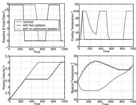
Fig. 3. Nominal and closed-loop simulation profiles of control and constraint variables:  $\Delta b_1 = -25\%$  and  $\Delta T_{in} = -10\text{ }^\circ\text{C}$  at  $t = 250$  sec
