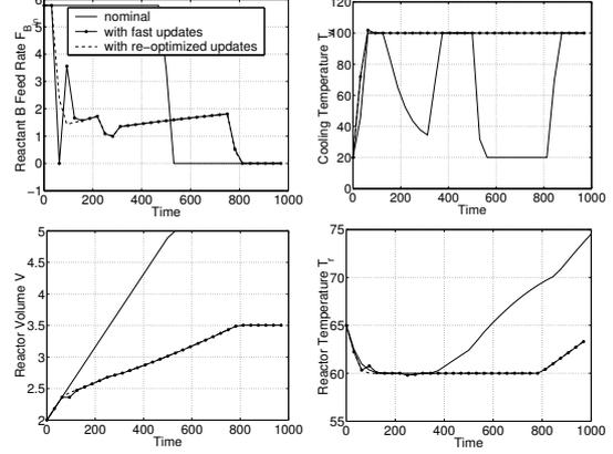
Fig. 2. Nominal and closed-loop simulation profiles of control and constraint variables:  $\Delta b_1 = +10\%$  and  $\Delta T_{in} = -10 \text{ }^\circ\text{C}$  at  $t=250$  sec
