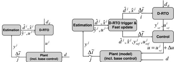
Fig. 1. Single level and two-level D-RTO
