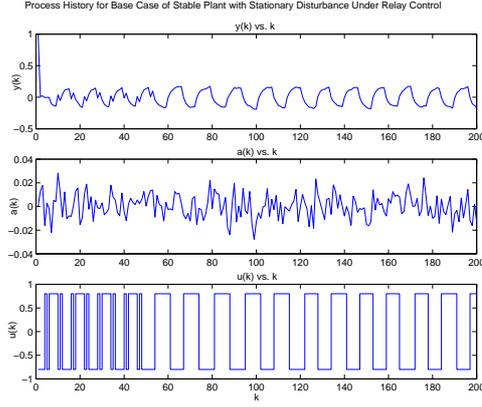
Fig. 3. Output and input history for base case of stable plant with stationary disturbance under relay control
