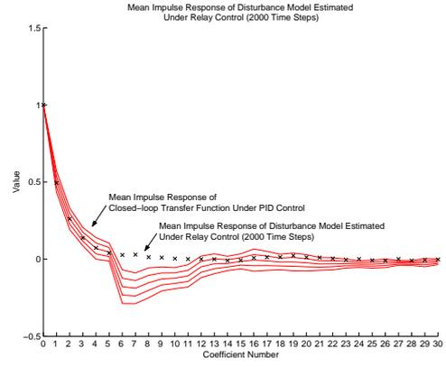
Fig. 5. Impulse response of the disturbance model estimated under relay control (2000 time steps)
