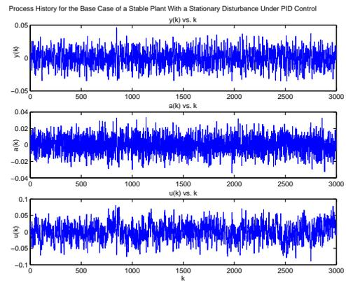
Fig. 1. Output, white noise, and input sequences for the stable plant with stationary disturbance under PID control
