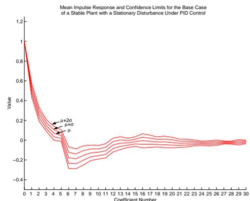
Fig. 2. Mean impulse response and its  $\sigma$  and  $2\sigma$  confidence limits for the stable plant with stationary disturbance under PID control
