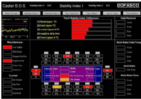
Fig. 3. Contribution plot screen of integrated monitoring system for #2 Continuous Caster
