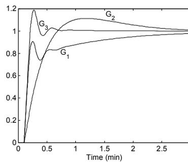
Fig. 6. Step response to setpoint change for  $G_1$ ,  $G_2$  and  $G_3$  models with MMA controller.
