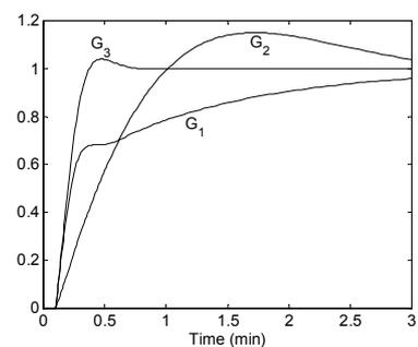
Fig. 7. Step response to setpoint change for  $G_1$ ,  $G_2$  and  $G_3$  models with SIMC controller.
