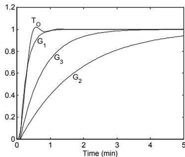
Fig. 4. Step responses for  $T_0$  and for  $G_1$ ,  $G_2$  and  $G_3$  models normalized by the static gain.
