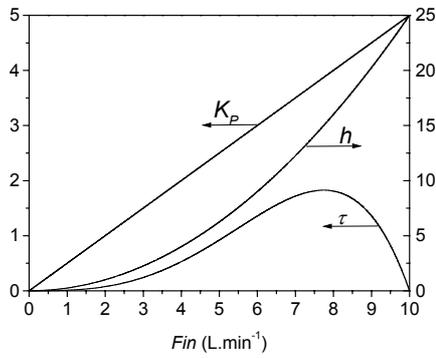
Fig. 3. Static gain ( $K_p$ ,  $\text{cm}\cdot\text{min}\cdot\text{L}^{-1}$ ), time constant model ( $\tau$ , min) and stationary height ( $h$ , cm), for the whole inlet flowrate ( $Fin$ ) range.
