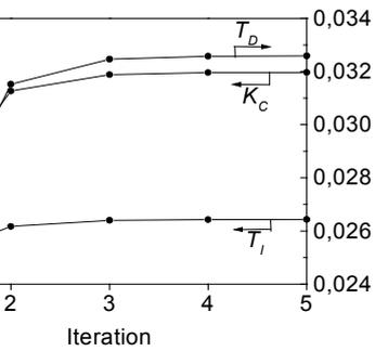
Fig. 5. Parameters convergence ( $K_C$ ,  $T_I$  and  $T_D$ ), for the iterations of the MMA optimization.
