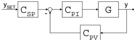
Fig. 1. The 2DOF feedback control configuration.
