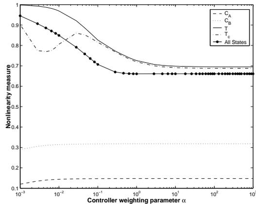
Fig. 3. Comparison of weighted OCL nonlinearities of CSTR model at sub-optimal operating point.
