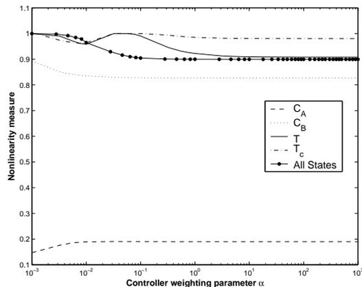
Fig. 4. Comparison of weighted OCL nonlinearities of CSTR model at optimal operating point.
