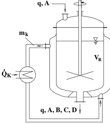
Fig. 1. Schematic of the CSTR.
