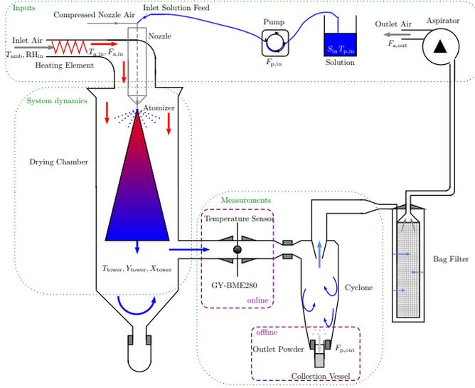
Fig. 1. Principle arrangement of a spray dryer, motivated by the case of the Mini Büchi B290 (similar to (Lepsien and Schaum, 2024a)).
