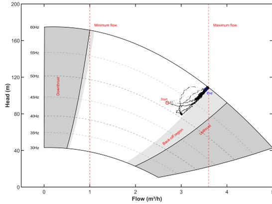
Fig. 7. Operational envelope of target MPC of scenario 03.
