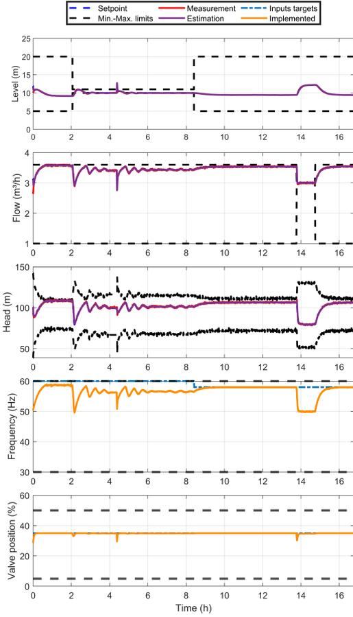
Fig. 4. Time responses target MPC of scenario 03.
