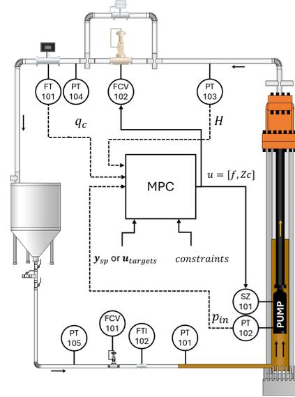
Fig. 1. LEA process diagram flow sheet.
