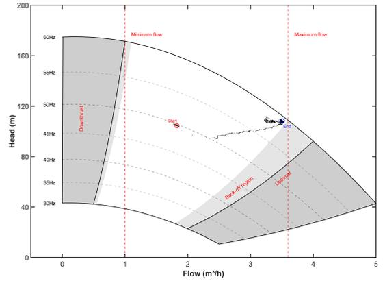
Fig. 6. Operational envelope standard MPC scenario 02.
