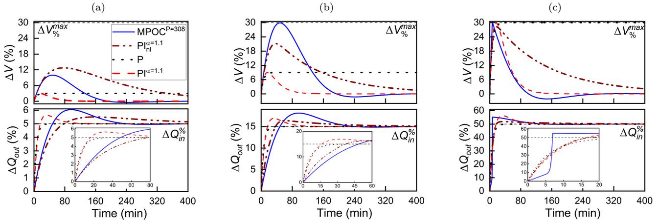
Fig. 2. Transient Response of  $Q_{out\%}$  and  $V_{\%}$  for step change in  $Q_{in\%}$  a) 5% b) 15% c) 50%
