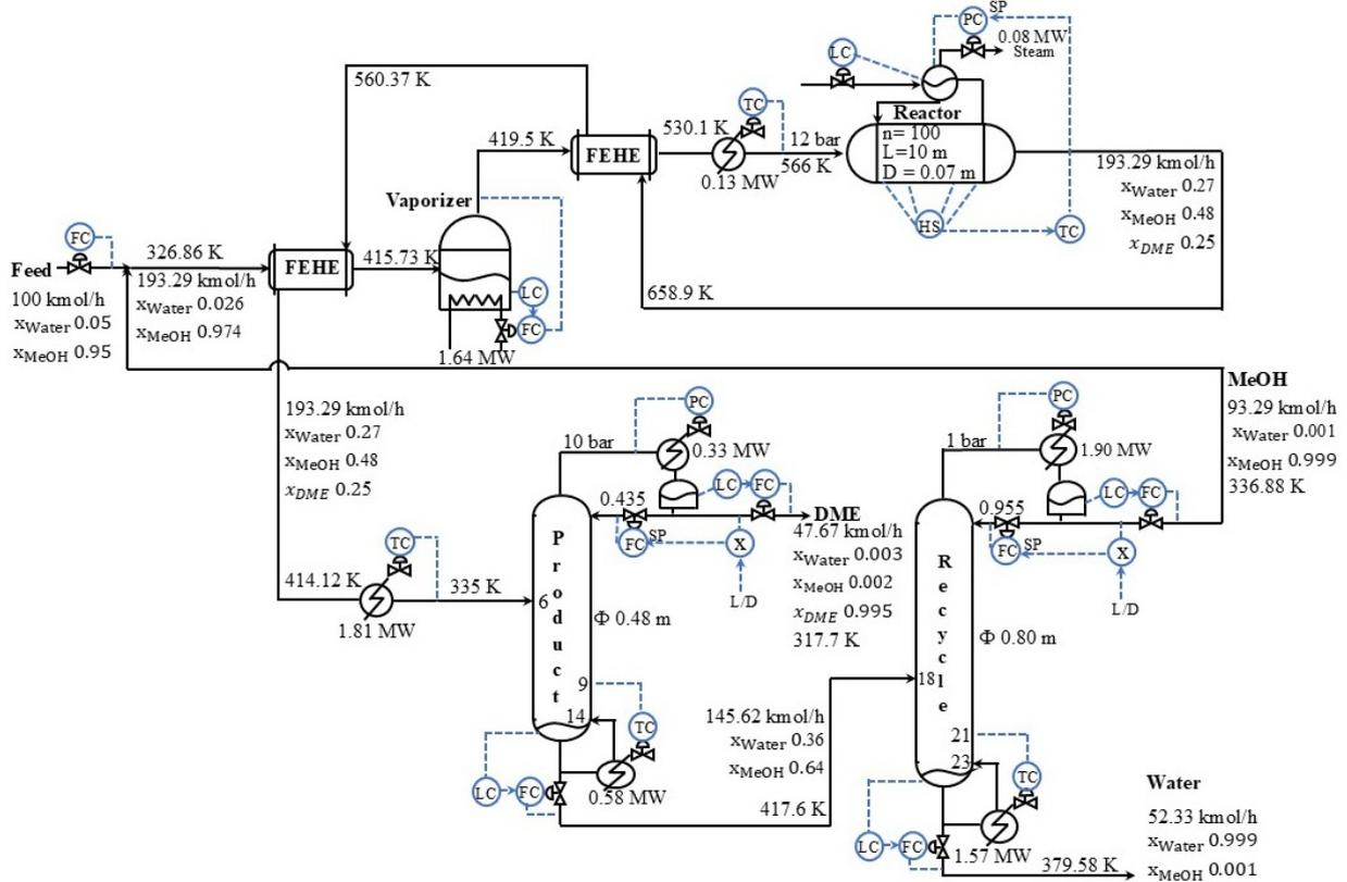
Fig. 3. Nominal design, operating condition and plantwide control structure of the MeOH dehydration process
