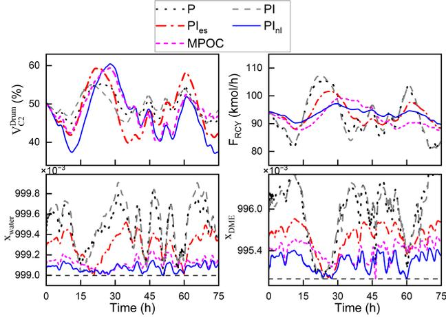
Fig. 4. Transient response of key parameters to time-series disturbance for MeOH dehydration process
