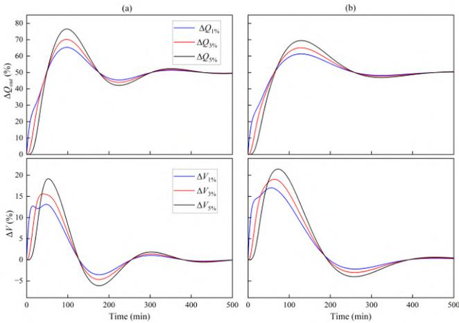
Fig. 3. Effect of  $\alpha$  on system transient response for PI LC
