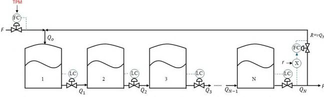
Fig. 1. Tanks-in-series process with recycle
