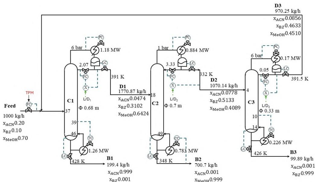
Fig. 7. Nominal design, operating condition (Zhu et al., 2016) and plantwide control structure (Luyben, 2017) of the MeOH-ACN-BZ process
