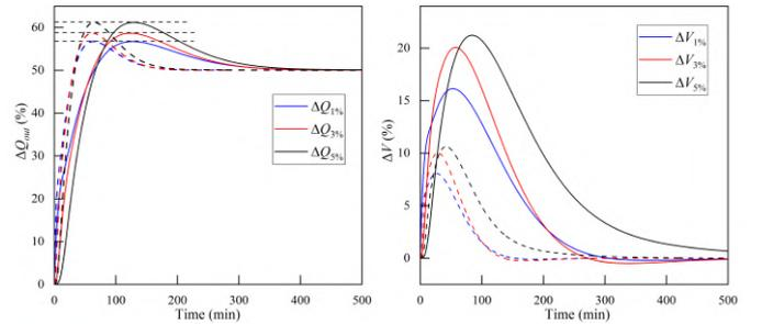
Fig. 4. Illustration of no change in flow overshoot for PI ALC at constant  $\alpha$
