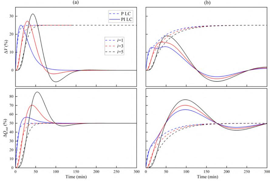
Fig. 2. System transient response to 50% step change in  $F\%$  with isolated tank ALC tuning
