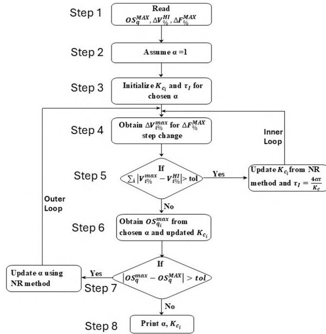
Fig. 5. Systematic detuning procedure of PI ALC
