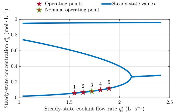
Fig. 1. Steady-state map of concentration  $c_A^s$  and coolant flow rate  $q_c^s$ .
