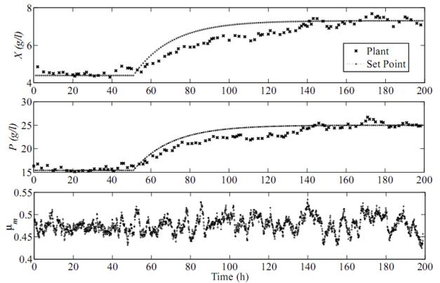
Fig. 5. Multi-rate servo control: Variation of controlled output and plant disturbance
