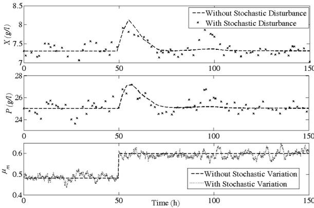
Fig. 4. Multi-rate regulatory control: Variation of controlled output and plant parameter ( $\mu_m$ )
