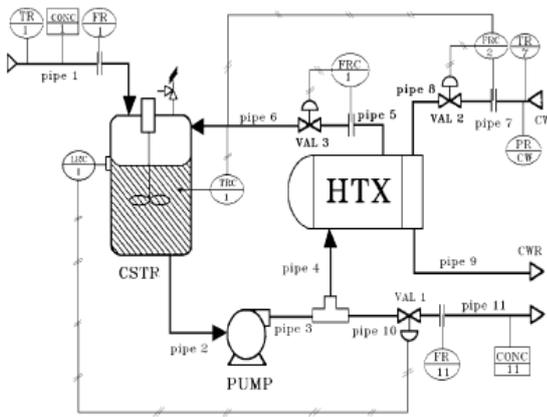
Fig. 2. Continuous Stirred Tank Reactor CSTR with recycle loop via Heat Exchanger HTX.
