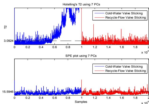
Fig. 4 Detection of Cool-Water and Recycle flow valve sticking using  $T^2$  and  $Q$  statistics of a PCA model.
