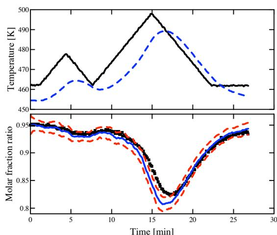
Figure 6. Analysis of the filter performance: (a) enforced wall temperature (solid line) and reactor temperature (dotted line); (b) CO estimated (or experimental) mole fraction concentration - in red continuous (or black dotted) plot – and estimate uncertainty (blue dotted) band in  $\pm$  standard deviation ( $\sigma$ ) wideness.
