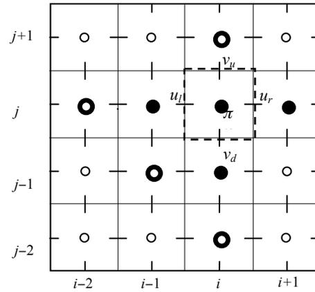
Figure 1. Arakawa-C grid with control volume and computational stencil for  $u > 0$  and  $v > 0$  (full points involved in definition of flux  $F_{i+1/2, j}$ ; empty, bold points involved in scheme for control volume).
