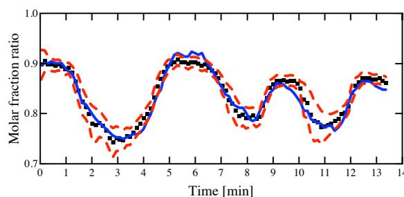
Figure 4. Kushner estimator functioning: CO estimated (or experimental) mole fraction ratio concentration - in red continuous (or black dotted) plot - and estimate uncertainty (blue dotted) band in  $\pm$  standard deviation ( $\sigma$ ) wideness.
