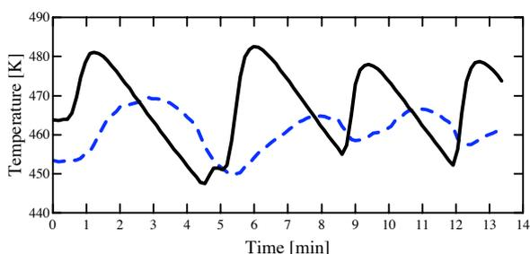
Figure 2. Enforced wall temperature (solid line) and reactor temperature (dotted line).
