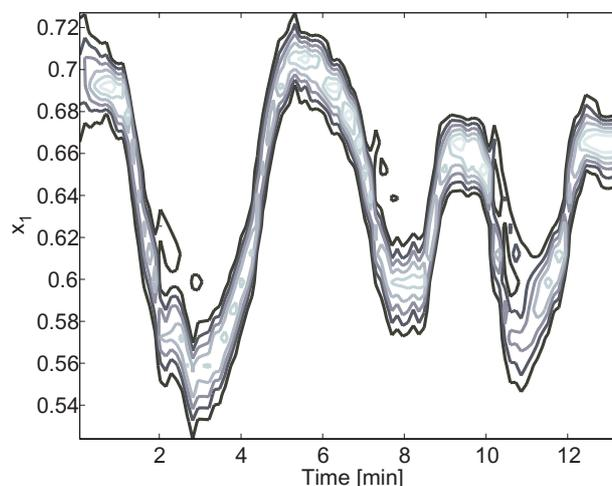
Figure 3. Kushner estimator functioning: PDF evolution in contour level form.
