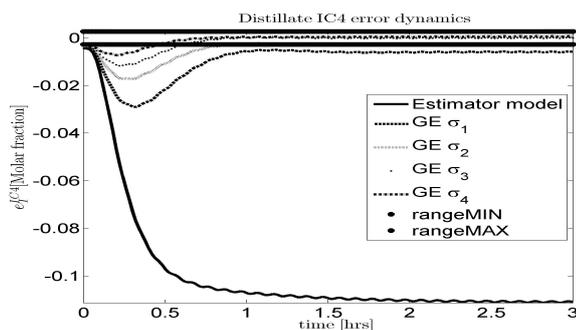
Fig. 3. Distillate IC4 composition error
