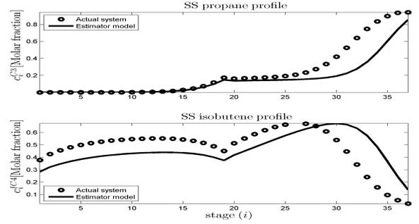
Fig. 1. SS composition profiles for 6-component system (2) (black circles) and 3-component estimator model (4) (black line)
