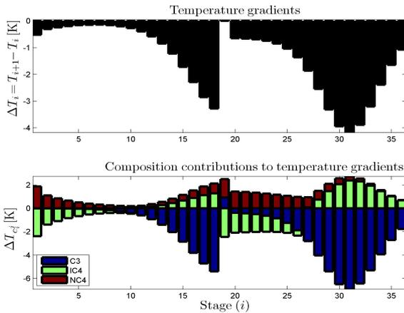
Fig. 2. SS temperature gradient and per-component contributions (10), based on the estimator model (4).
